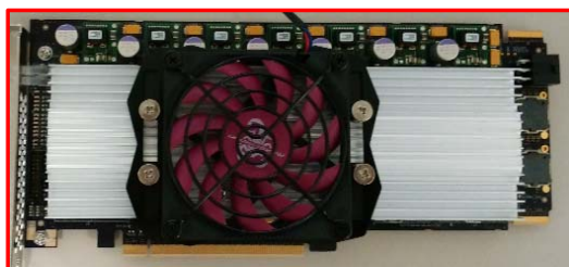
MISD style Dataflow pipeline on FPGA (Maxeler Galava card)
